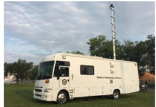
Figure 2. Mobile Air Monitoring Laboratory (MAML). Source: Shane Taylor
