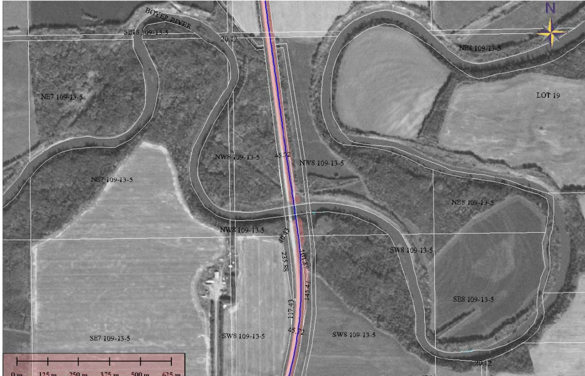
Figure 10: Recommended Downstream Alignment – Grading Extents & Existing ROW
