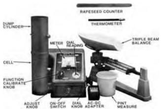
Figure 1. Detailed View of Labtronics 919 Grain Moisture Meter.
