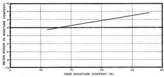
Figure 4. Deviations of Meter Readings for the Labtronics 919 in Oats.
