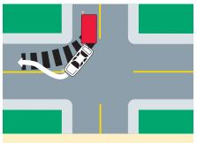
Turning right when towing a trailer - note the path of vehicle and trailer wheels.
