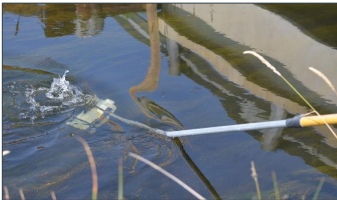
Water sampling from an irrigation canal during the Irrigation District Water Quality project
