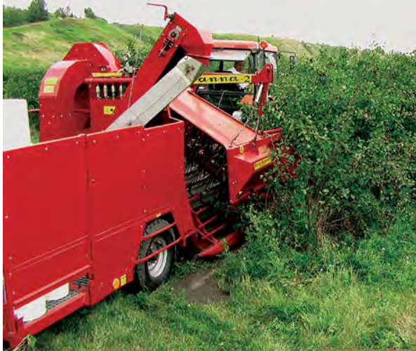
Figure 98. Sideways Joanna harvester enters row; the harvester is beginning a new row at The Saskatoon Farm, Dewinton, Alberta. The plastic mulch is also visible, but the harvester will not damage the mulch if it is properly installed. Photo: Bob Bors
