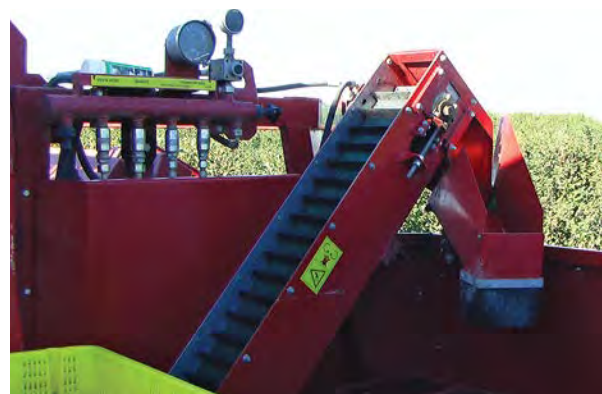
Harvested fruit travels up the stepped escalator, and the fruit tips into chute and falls into flats. Image also shows the mechanisms (below gauge) for adjusting vibration and speed, etc.
