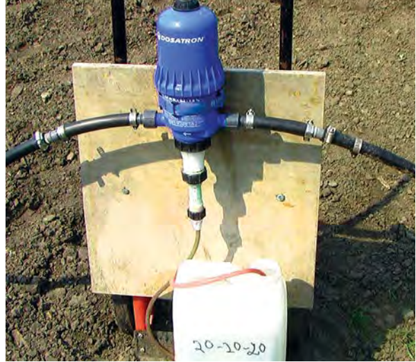
Figure 14. Inline fertilizer drip system – fertilizer is distributed to the plants through the drip line watering system. Photo: Bob Bors
