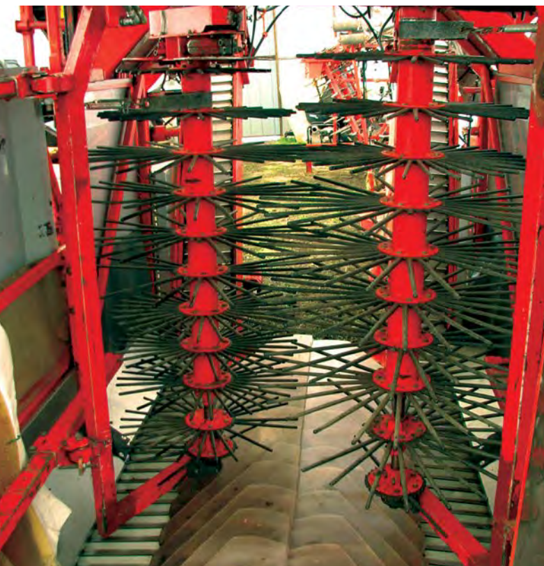
Figure 96. Upright, over-the-row harvester from front; the fish plates are the sliding plates on the bottom over opening below tines. Photo: Robert Spencer
