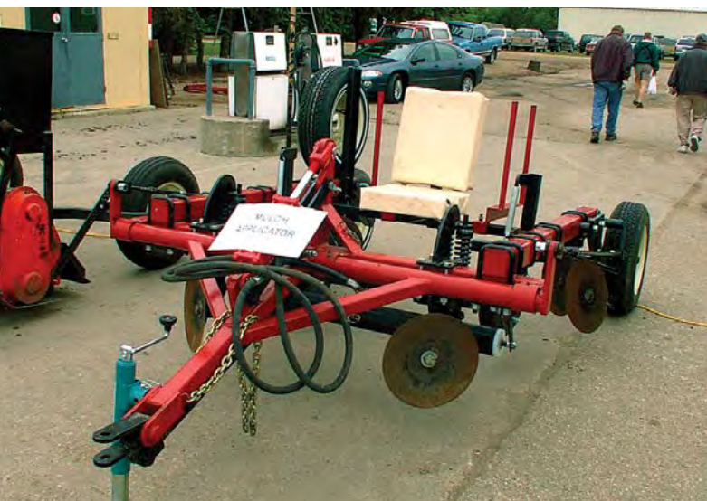
Figure 20. This plastic mulch applicator can also mechanically plant small plugs simultaneously. Photo: Bob Bors
