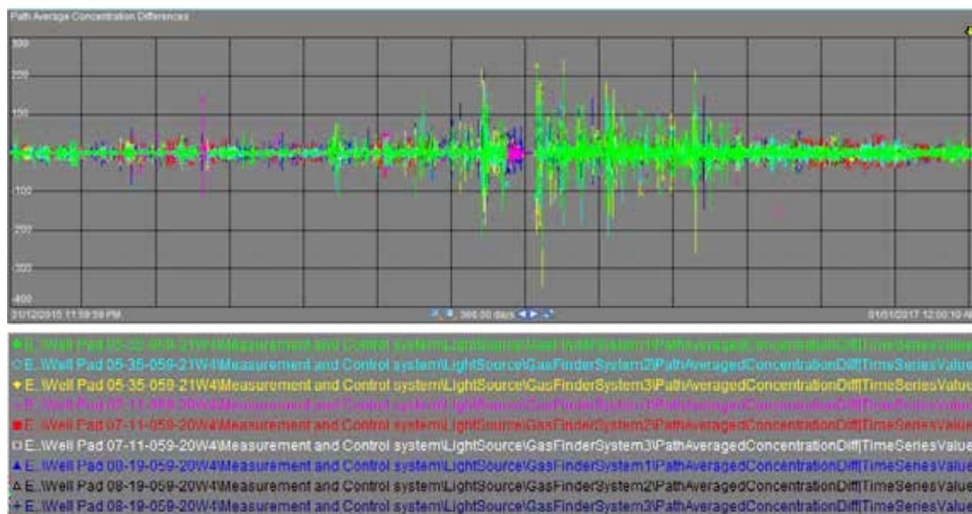
Figure 4-2: Time series plot of path averaged CO 2 concentrations difference [ppm] recorded at pads 5-35, 7-11 and 8-19 between June 2015 and December 2016.
