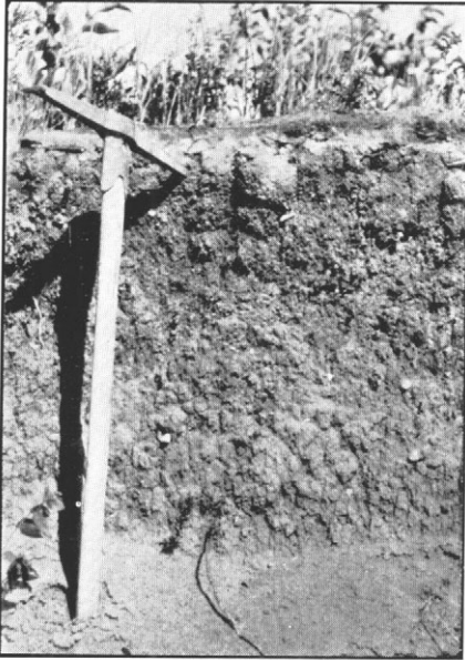
Fig. 1 — Incipient podsol soil profile. Note heavy granular subsoil, typical of much of this area, below the thin light colored leached layer. (See p. 18.)
