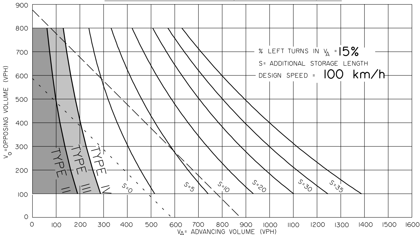
FIGURE D-7.6-6b WARRANTS FOR LEFT TURN TREATMENT AND STORAGE REQUIREMENTS FOR TWO-LANE HIGHWAYS DESIGN SPEED 100 KM/H, LEFT TURN 15%, 20%
