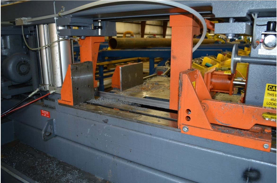
Figure 5 shows a close up of the bandsaw in the “down” position with the cut pipe removed.
