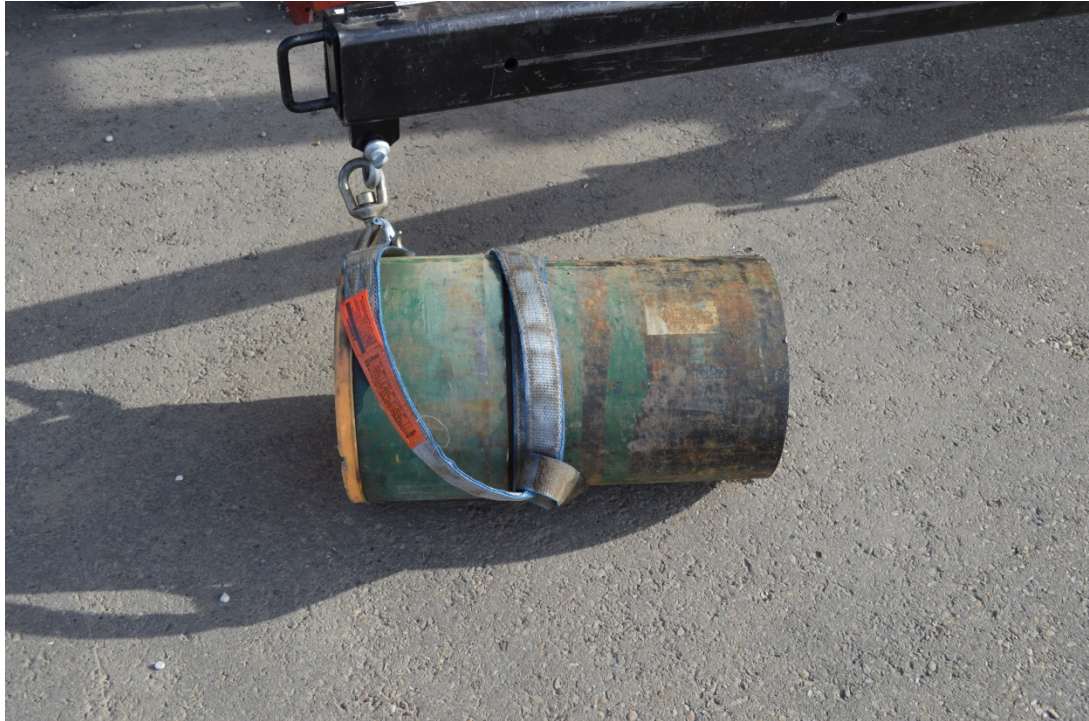
Figure 6 shows the cut piece of pipe that was removed from the bandsaw that the production worker was holding up
