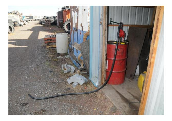
Photograph 5 – View from the west of the shed, 205 liter drum of gasoline with barrel pump, and the hose used to refuel the Toyota, Model 5FG15 forklift. The hose extended 1.62 meters outside of the shed.
