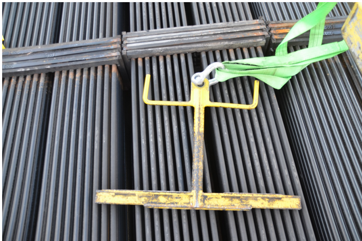
Figure 4. T-Bar resting on sucker rod bundles. Photo taken at Arrow Reload yard.
