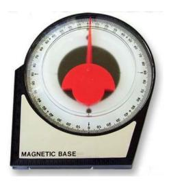
An Inclinometer has a magnetic base. This makes it ideal for attaching to brake discs on a motorcycle.
