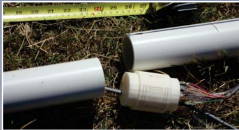
Point velocity probe used to measure groundwater velocity and direction at the centimetre scale.
