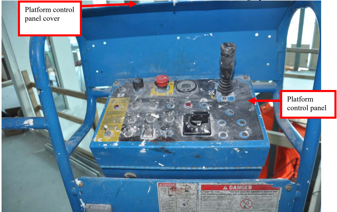
Photograph 4 – Shows the Genie lift platform with the platform control panel and cover that the POS worker was utilizing in the lift platform between the second floor mezzanine and ceiling bulkhead when the POS worker was found pinned by the neck between the ceiling bulkhead and the platform control panel.
