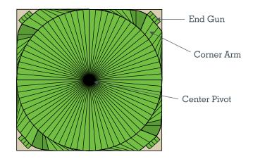
Figure 1. Schematic for path of corner arm centre pivot irrigation system. Source: Image provided by Valley Irrigation
