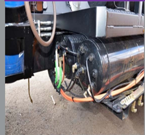
Air tank check valve
