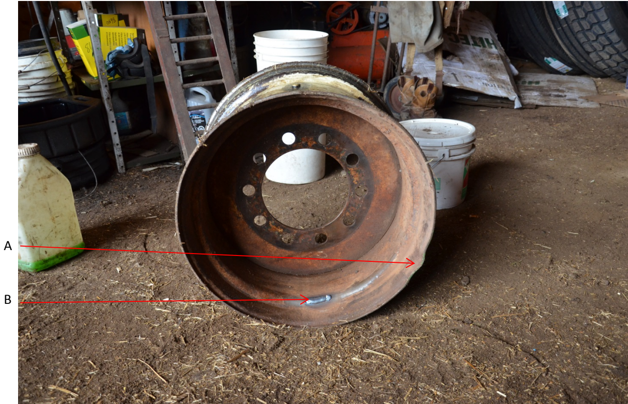
Figure 3 – Rim from the incident A – Damage caused by the incident B – The weld
