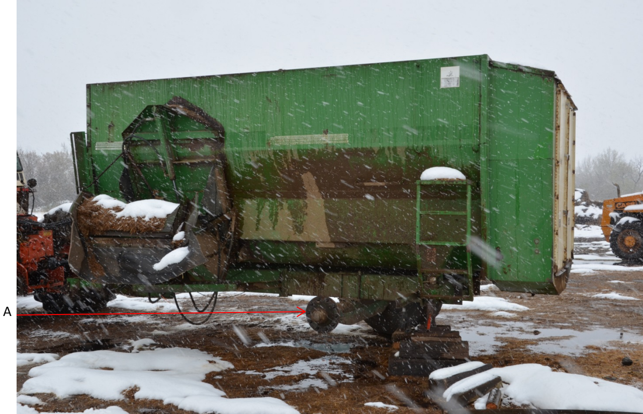
Figure 4 – Henke wagon with the tire assembly removed
