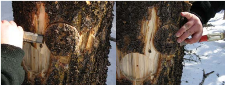
Figure 6. Remove wood ¼ inch away from hole saw cut, loosen disk from sides and wedge out with inverted chisel.
