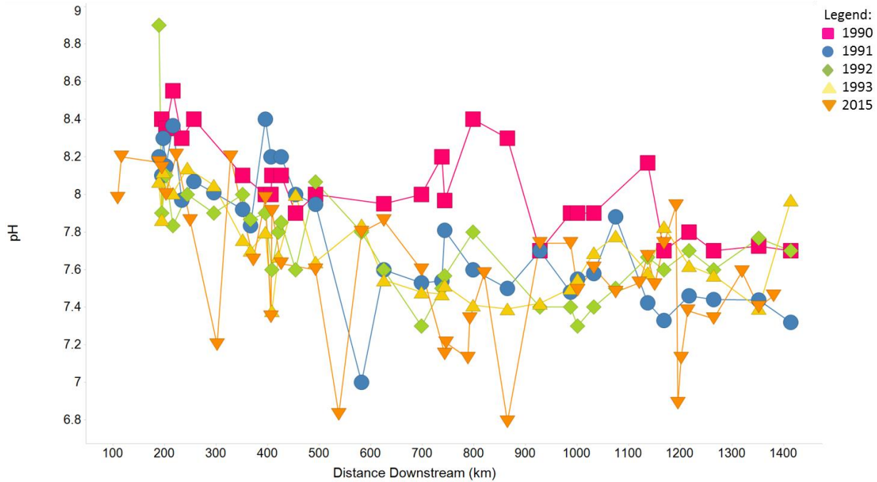
Figure 12. Comparison of pH measured in the Athabasca River during the winter synoptic surveys from 1990-1993 and 2015.
