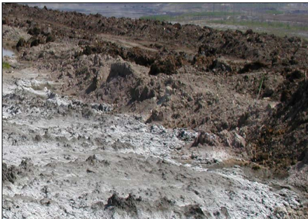
Image 15. Lower slope of a saline sodic overburden substrate displaying a high risk salinity constraint.
