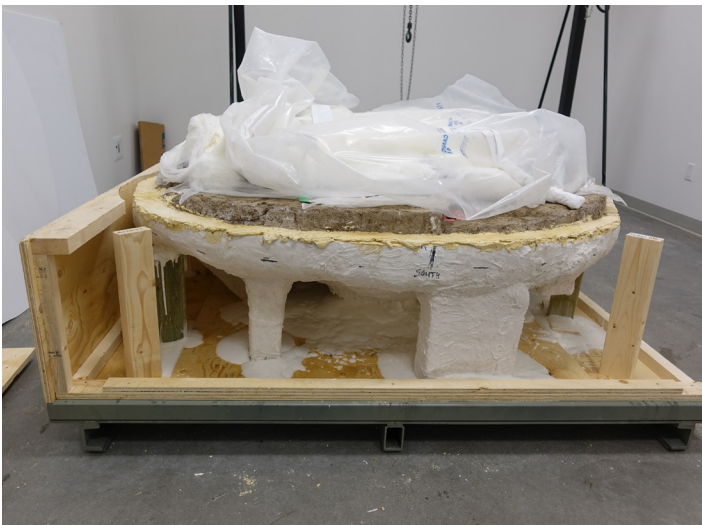
Figure 26. Detail of fabrication of display case assembly. Upright boards are supports for plywood apron.
