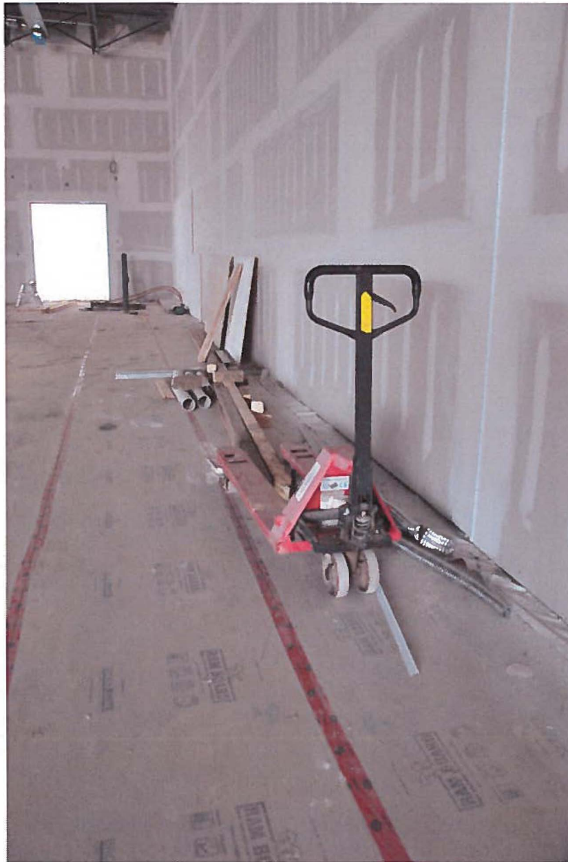
Photograph #2 Shippers Supply pallet jack .52 m x 1.22 m, weight capacity 2494 kg.
