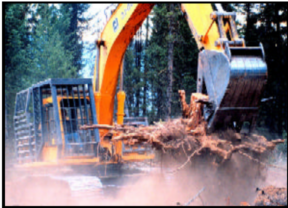
Excavator pulling Armillaria-infected stump.
