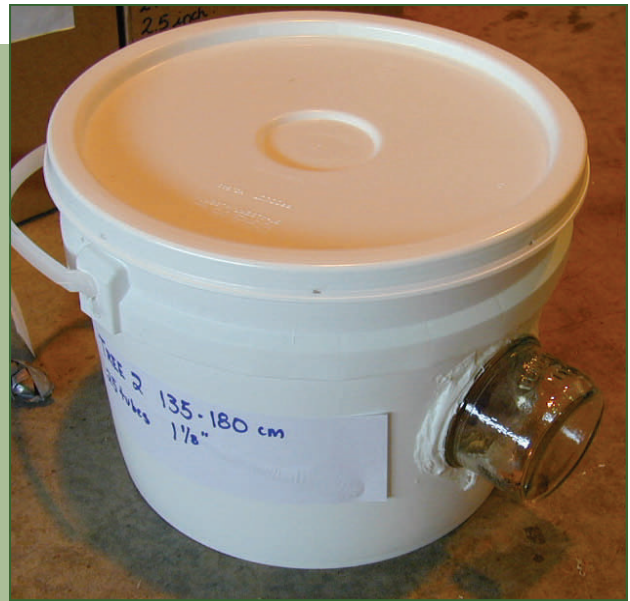
MPB emergence trap containing 1 1/8 " wood chips.
