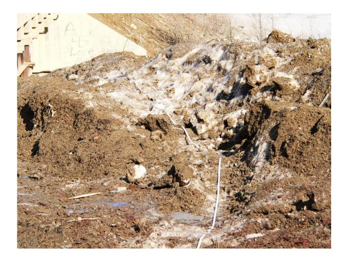
Photograph #3 Shows the track made in the snow bank by the passenger side wheels of the Foreman's truck. The tape shows the wheel track.
