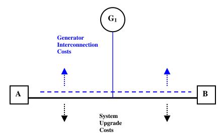
Local "system" upgrades typically include items such as changes to stations A and B (i.e. circuit breaker change-outs, protection upgrades), reconductoring of Line A-B, or other modifications to the local system to accommodate the generator. These costs will be considered "system" costs and will not be recovered specifically from a particular generator but will be treated like all other system costs.
