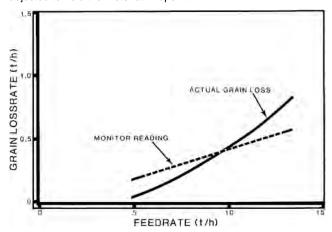
**FIGURE 4.** Comparison of Monitor Reading to Actual Combine Lossrate in a Field of Bonanza Barley.
