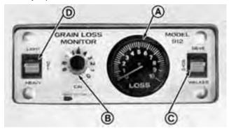
FIGURE 3. Control Box: (A) Loss Meter, (B) Calibration Control, (C) Sensor Selector, (D) Sensitivity Control and Power Switch.
