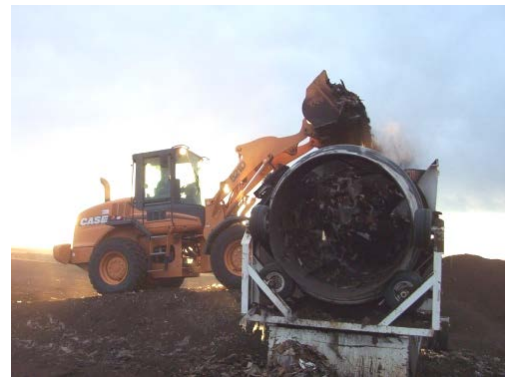
Photo 3.36. Front-end loader feeding a portable trommel screen Source: Scott Gamble
