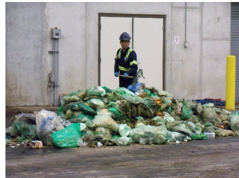
Photo 4.2. Manually inspecting feedstocks for contaminants
