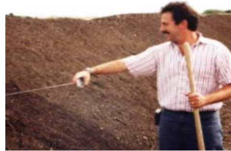
Photo 4.19. Measuring windrow temperatures with a bimetal thermometer
