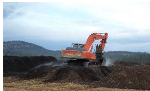
Photo 4.8. Turning a windrow with a tracked excavator
