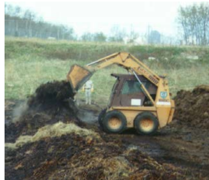
Photo 3.28. Skid-steer loader Source: Scott Gamble
