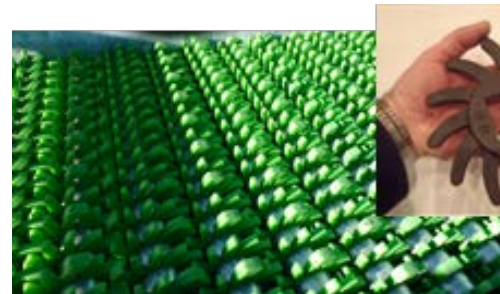
Photo 3.37. Top view of star screen deck and side view of individual star Source: CH2M
