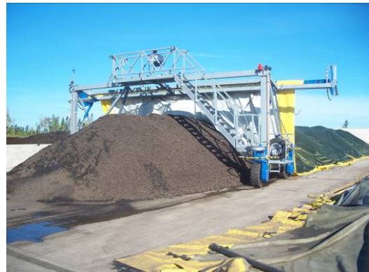
Photo 3.15. Mobile tarp winder used to place and remove compost covers
