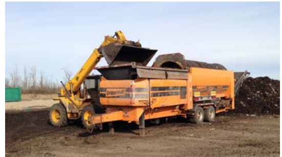
Photo 4.10. Screening compost with a portable trommel
