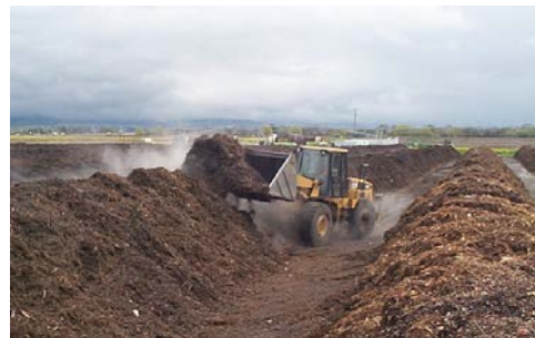
Photo 4.9. Turning a windrow with a front-end loader
