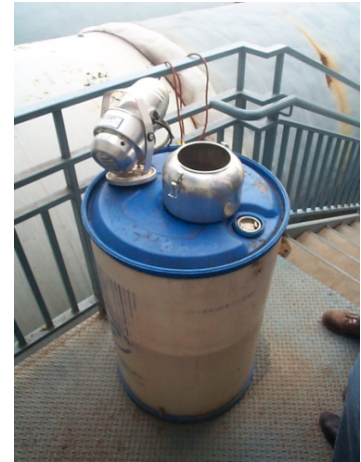
Photo 4.34. Portable mist sprayer for masking agents used at a composting facility.
