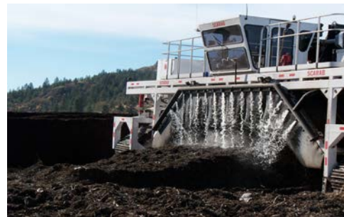
Photo 4.17. Spraying water onto a windrow during turning Source: CH2M
