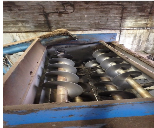
Photo 3.34. Horizontal auger mixer Source: CH2M
