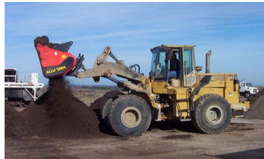
Photo 3.31. ALLU bucket on a front-end loader
