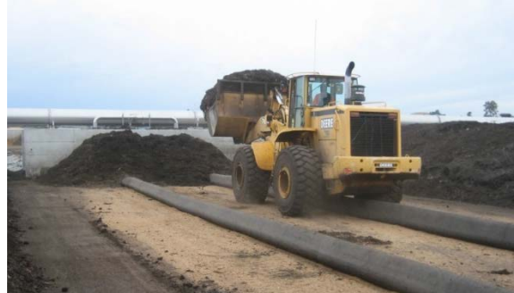
Photo 4.6. Using a front-end loader to build a pile in an ASP system
