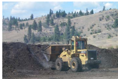
Photo 3.30. Front-end loader with an oversized bucket Source: CH2M
