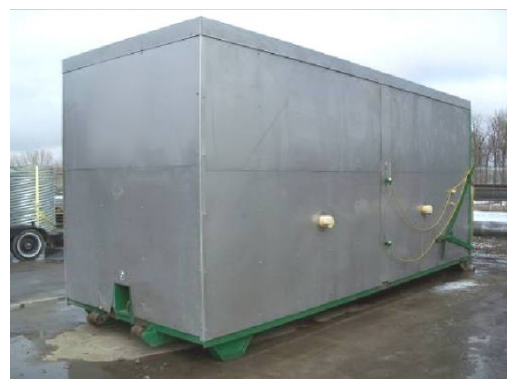
Photo 3.21. Static container composting system
