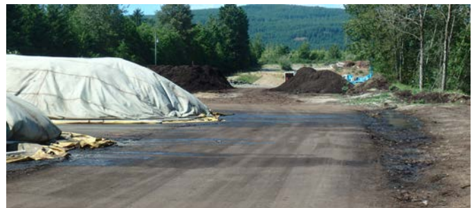
Photo 4.35. Runoff and leachate from composting facilities can have high BOD and contain other contaminants, and should be contained
