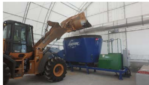
Photo 3.35. Loading a vertical auger mixer Source: CH2M
