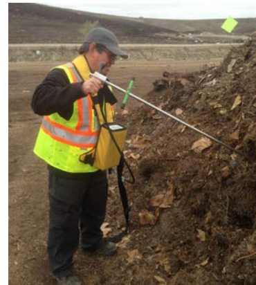
Photo 4.21. Measuring oxygen concentration in a windrow
