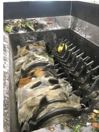
Photo 3.33. Shear shredder Source: CH2M
