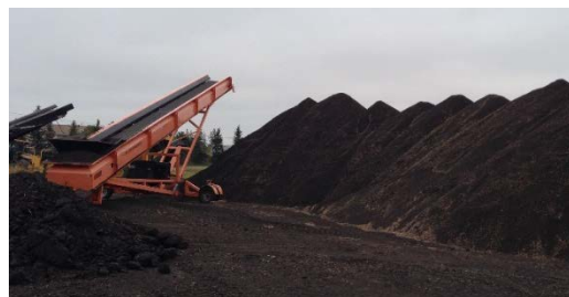
Photo 3.41. Stacking conveyors allow tall piles to be made, without having to drive equipment on top of the material
