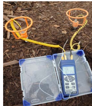
Photo 4.20. Using a datalogger to collect temperatures in an ASP
