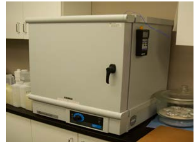
Photo 4.23. Oven used for measuring moisture content in a lab
