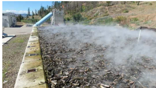
Photo 4.31. Biofilters are commonly used to treat odours from composting systems
