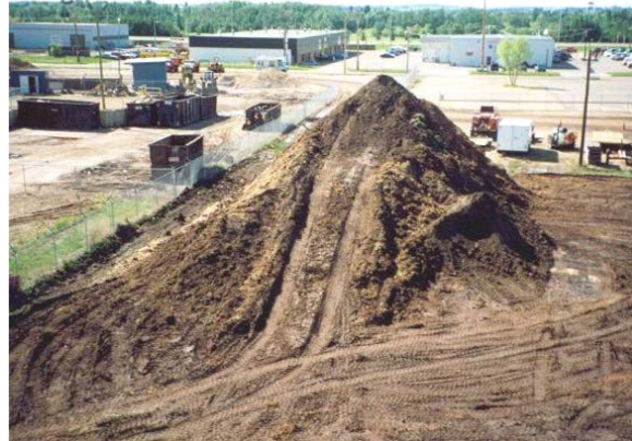
Photo 3.3. Overly-large static pile that has been compacted by heavy equipment
