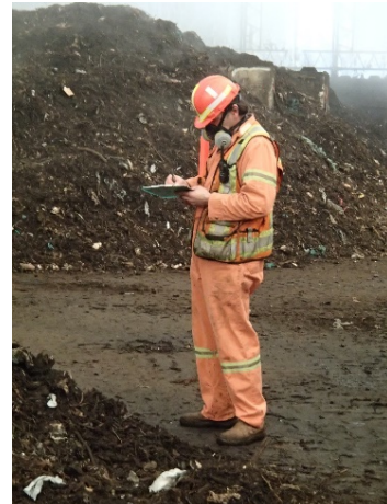
Photo 7.11. Employee wearing PPE and Respiratory Protective Equipment in an enclosed composting building
