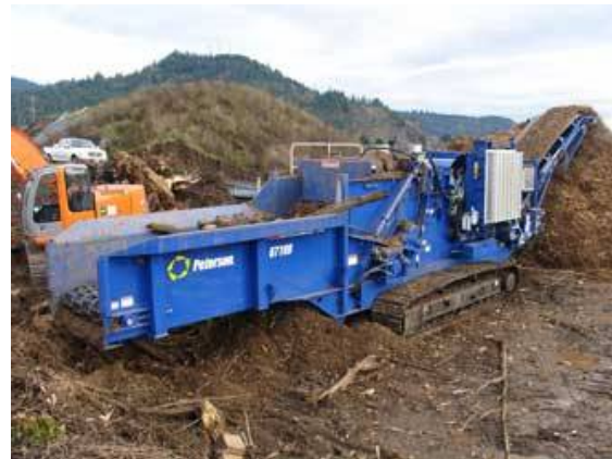
Photo 3.32. Horizontal grinder Source: CH2M
