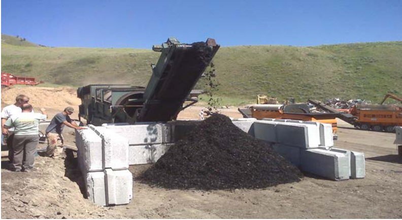
Photo 1.10. Producing colored mulch from ground wood waste
