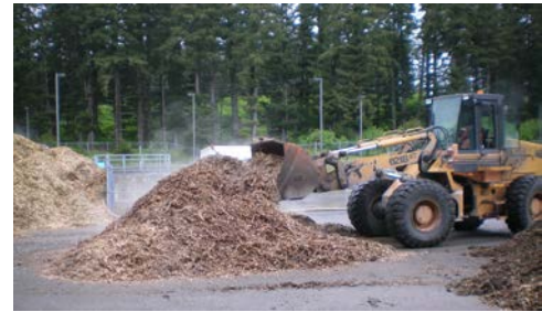
Photo 4.3. Using a front-end loader to mix feedstocks and amendments
