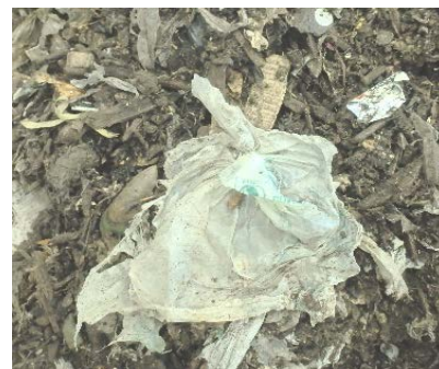
Photo 2.6. Compostable plastic liner bag after three weeks of active composting Source: CH2M
