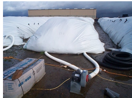
Photo 3.14. Composting system using polyethylene covers Source: Scott Gamble
