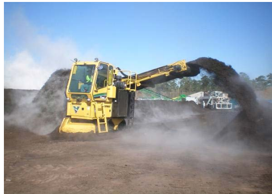
Photo 3.8. Self-propelled mass bed turner with discharge conveyor
