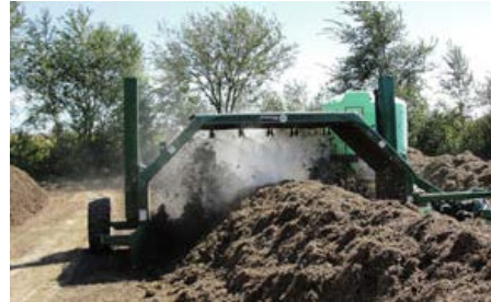
Photo 2.9. Adding water to a windrow during turning
