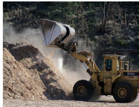
Photo 3.29. Roll-out bucket on a front-end loader Source: CH2M
