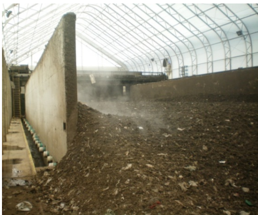
Photo 3.19. Agitated bay system in Lunenburg, NS viewed from discharge end of bay
