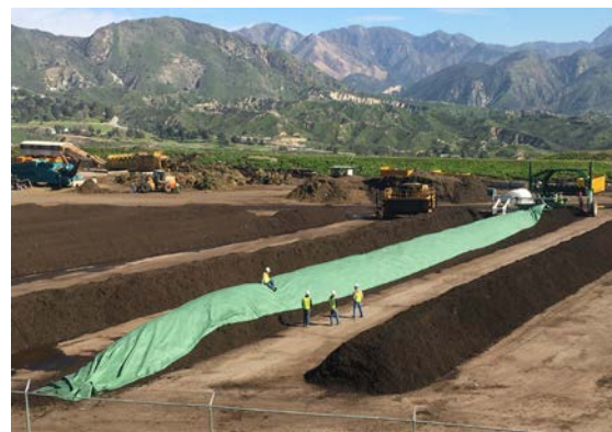
Photo 4.29. Winder system placing a tarp over a long windrow
