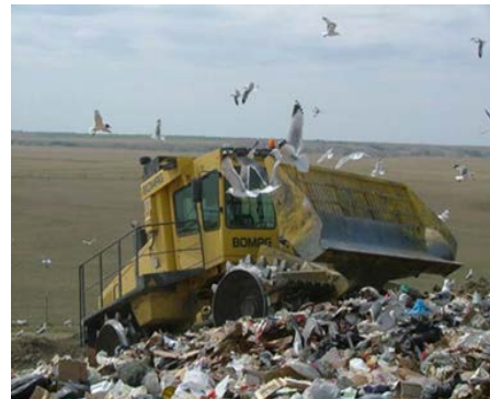
Photo 1.4. Compactor at a landfill Source: JL Technical Services
