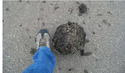
Photo 4.5. Over-mixing biosolids can lead to large “sludge balls”
