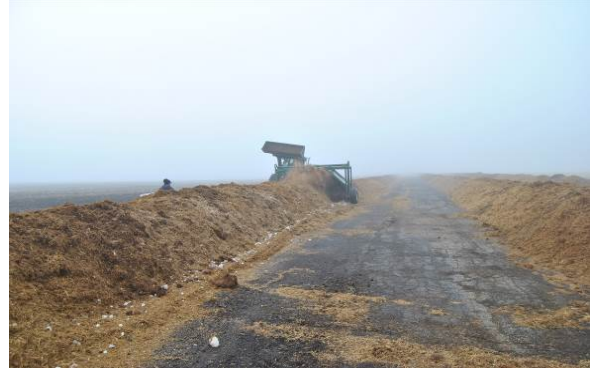
Photo 1.2. Windrow composting Source: JL Technical Services
