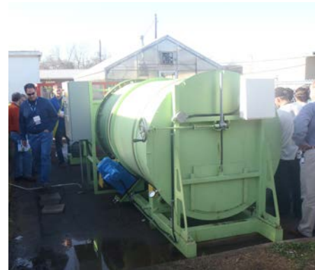
Photo 3.27. Small-scale drum composting system
