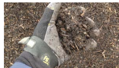
Photo 4.22. Judging moisture content with a squeeze test
