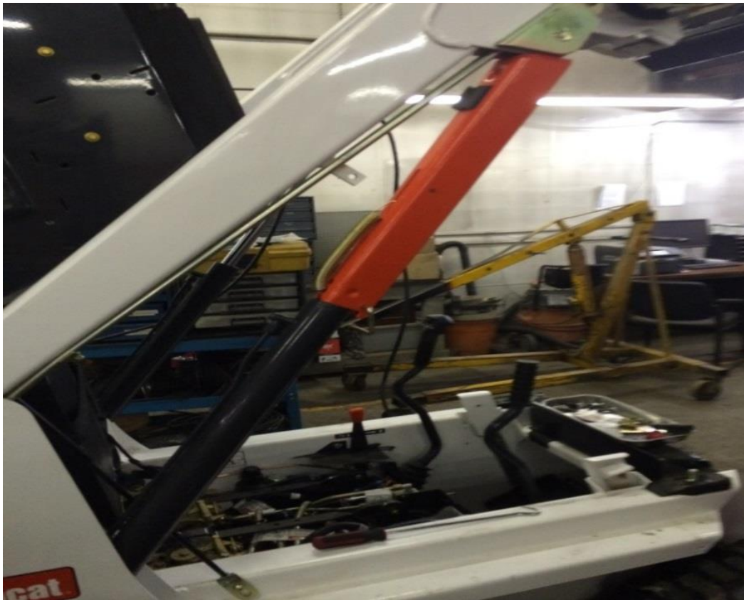
Figure 5. An example of the lift arm support in position holding the boom while the lift-arms are raised.
