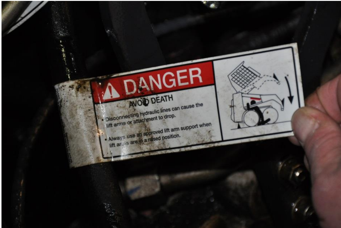
Figure 8. A tag within the cab of the skid-steer indicated that “disconnecting hydraulic lines can cause the lift arms or attachment to drop.”
