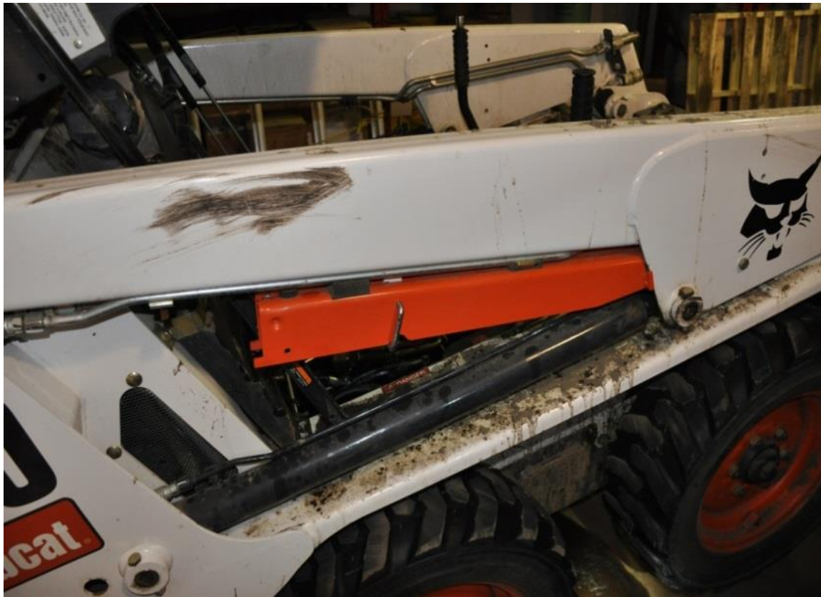
Figure 4. The skid-steer lift-arm support was still in the cradle of the boom while the lift-arm with the bucket attached were raised.
