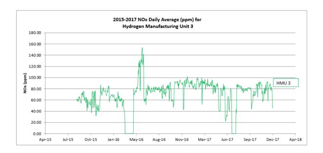
We believe the NOx emissions are trending up since the start-up of Quest partially due to the fouling of the burners, especially in the axial region. This would cause more gas hold-up which would result in more NOx being produced. The amount of NOx is also related to the heating value of the burner fuel gas source and the amount of CH4 in that stream, which follow the same trend as the amount of NOx emitted.
